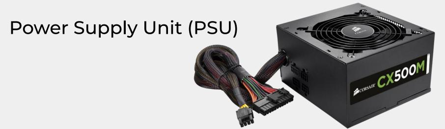
A *power supply unit* (or PSU) converts mains AC to low-voltage regulated DC power for the internal components of a computer. Modern personal computers universally use switched-mode power supplies. Some power supplies have a manual switch for selecting input voltage, while others automatically adapt to the mains voltage. (wp)
